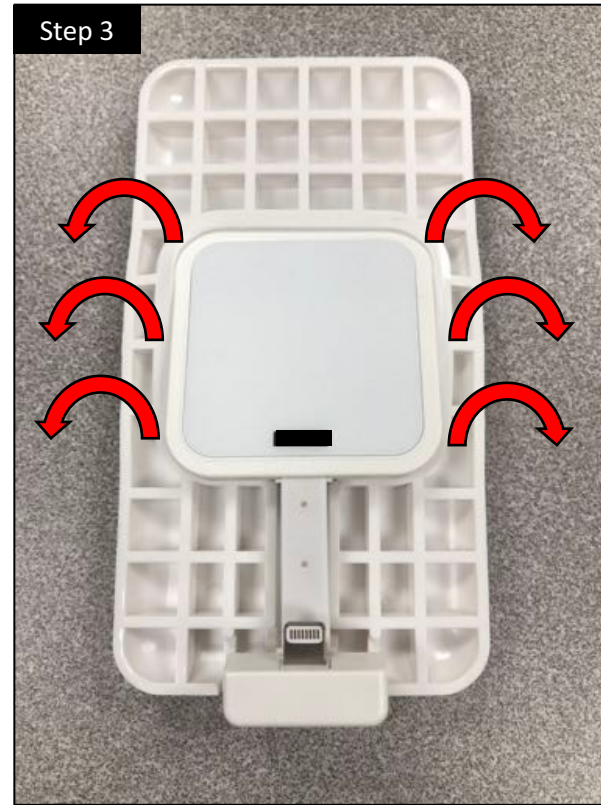
Slightly bend the Spacer to fit the AsRing+ into place one side at a time.
